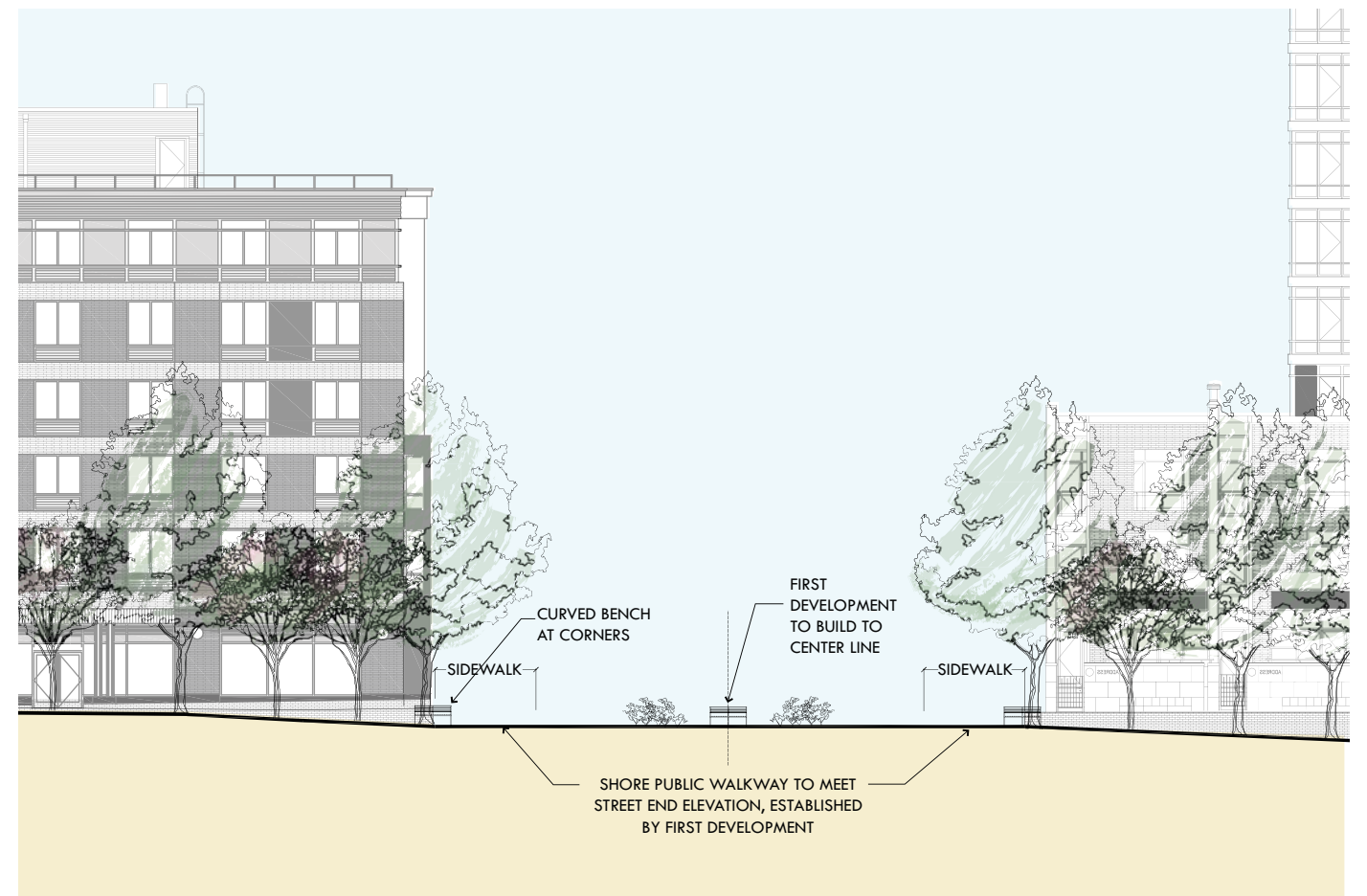
FIGURE 4-6: CROSS SECTION OF STREET/UPLAND CONNECTION INTERSECTION. ARCHITECTURAL ELEVATIONS, COURTESY OF FXFOWLE ARCHITECTS, PC.
