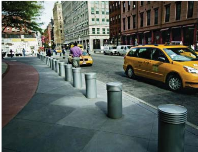
FIGURE 6-50: STANDARD STAINLESS STEEL BOLLARD
