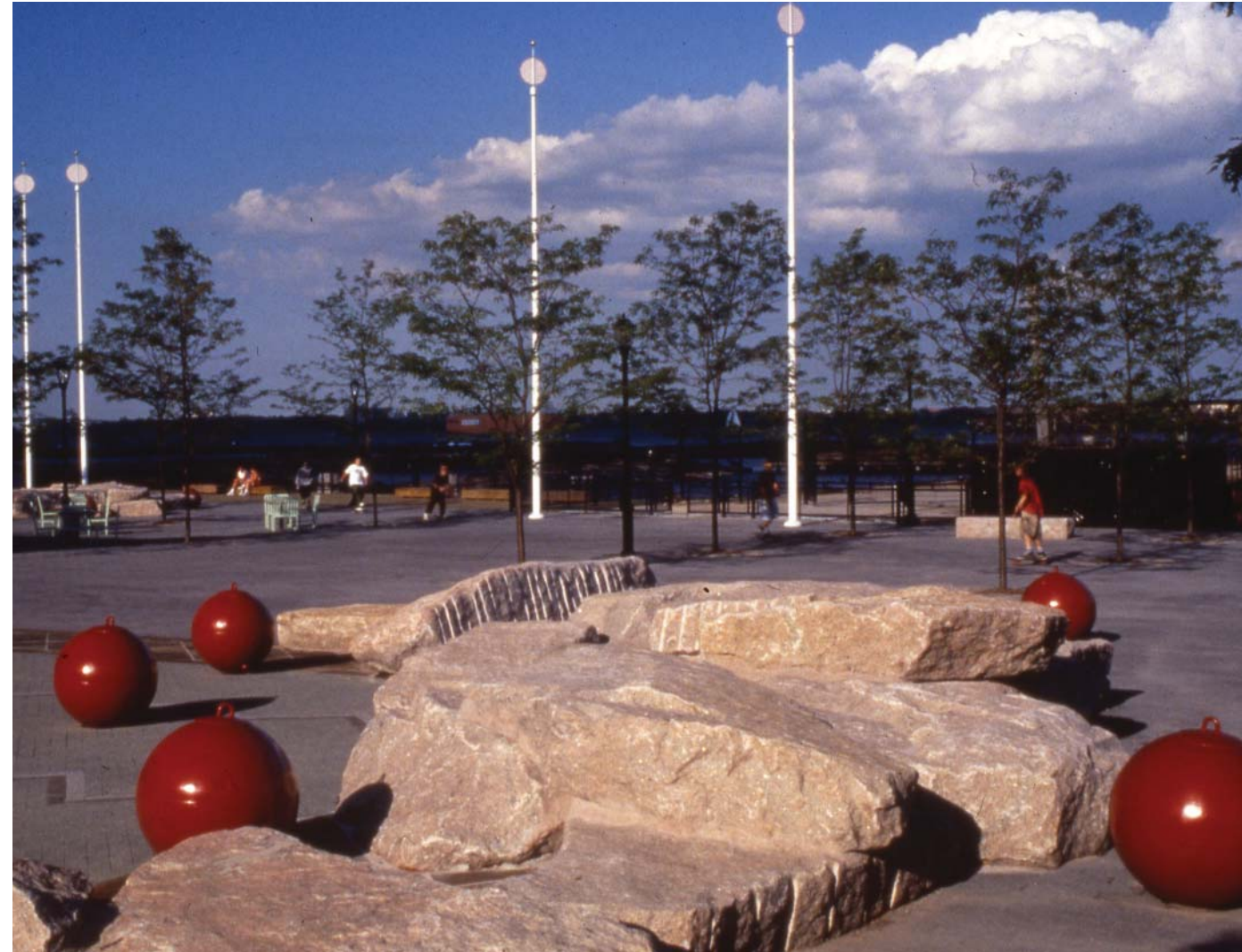
FIGURE 6-51: ALTERNATIVE BOLLARD MATERIALS
