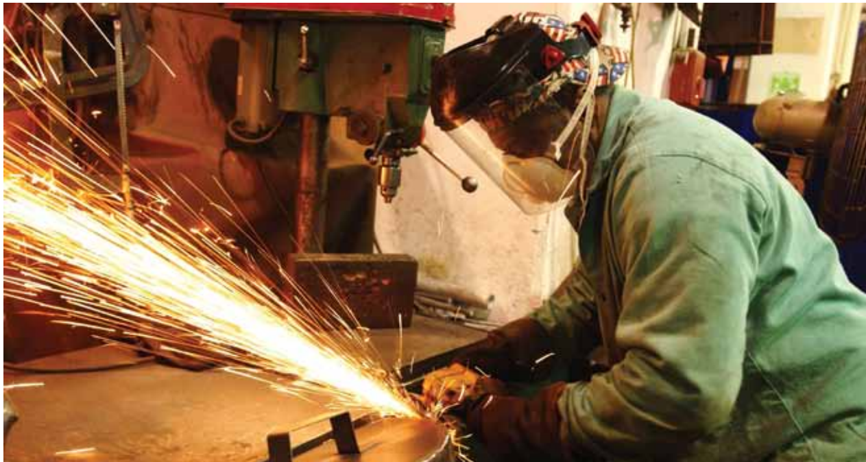
Above: A Parks blacksmith grinds the tub of a BBQ grill for a park. Photo Credit: Spencer Tucker.
