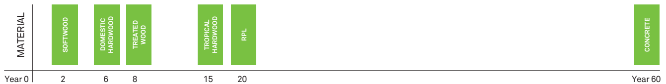
ESTIMATED SERVICE LIFE FOR DECKING OPTIONS ON THE CONEY ISLAND BOARDWALK AT BRIGHTON BEACH
