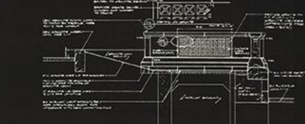
42nd Street Plinth Section/Elevation Scale: 1/4" = 1'-0"
